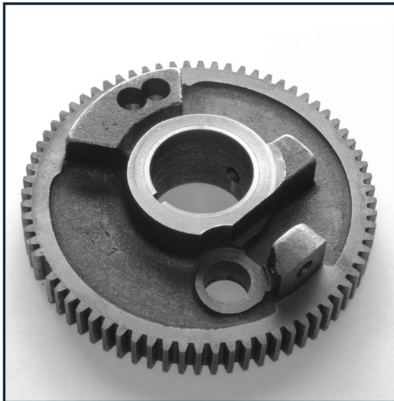
Figure 16: Damaged cast gear subject to reverse engineering
